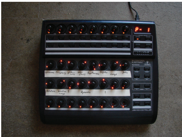
Figure 3 Knob-box MIDI Controller used in LiveScore.
